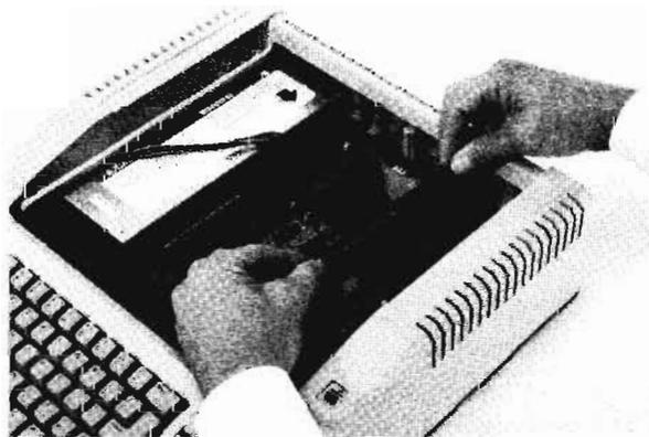
**Figure 1-6** Inserting the card in the slot
